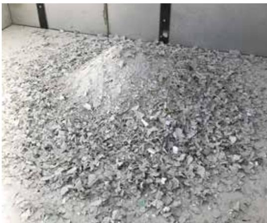
2 Gypsum waste after initial shredding in the BHS pre-shredder: The procedure allows for reliably sorting of metal parts
