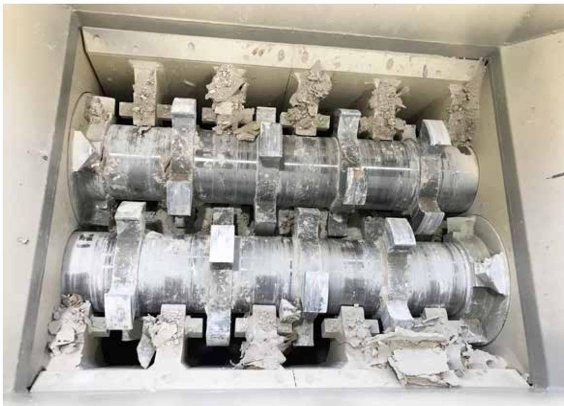
1 The two shafts of the pre-shredder of type VSR are equipped with shredding tools that can easily handle impurities in the gypsum waste
